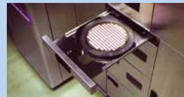
Inspection stage, used for checking the results of dicing
